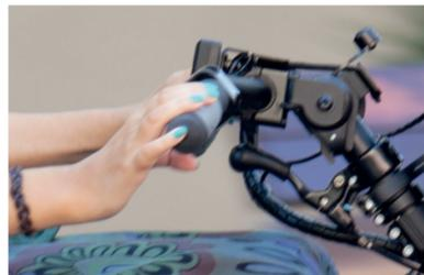
The **quadriplegic** version includes a **handlebar without levers** for smooth movements when braking and accelerating.
